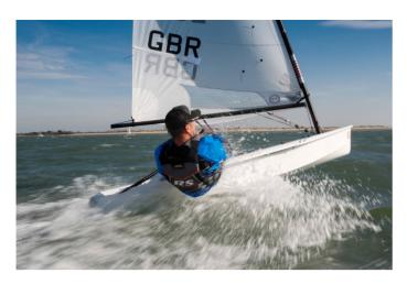
The company found through testing that a 4 m long hull would be long enough to support the larger helmsman, without being too much of a handful for small sailors to launch and recover.
